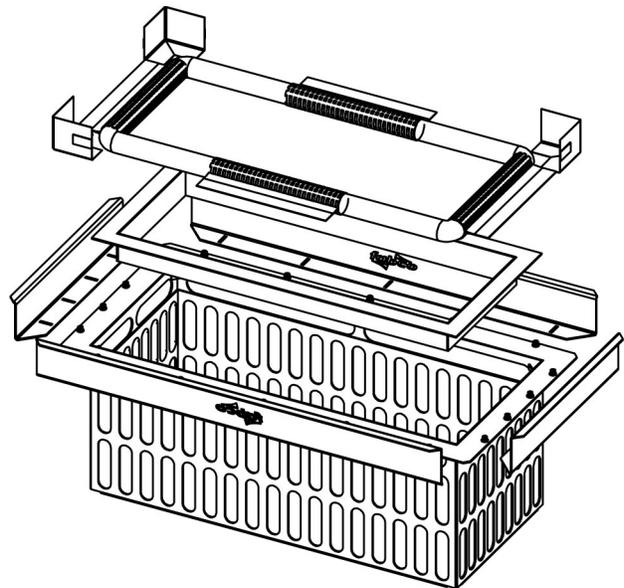
The **Fabco ScreenBox** will deliver assembled and consists of the components designated below. The Frame/Flange system uses a sliding flange that provides 1.5" of adjustability on all four sides of the frame.
